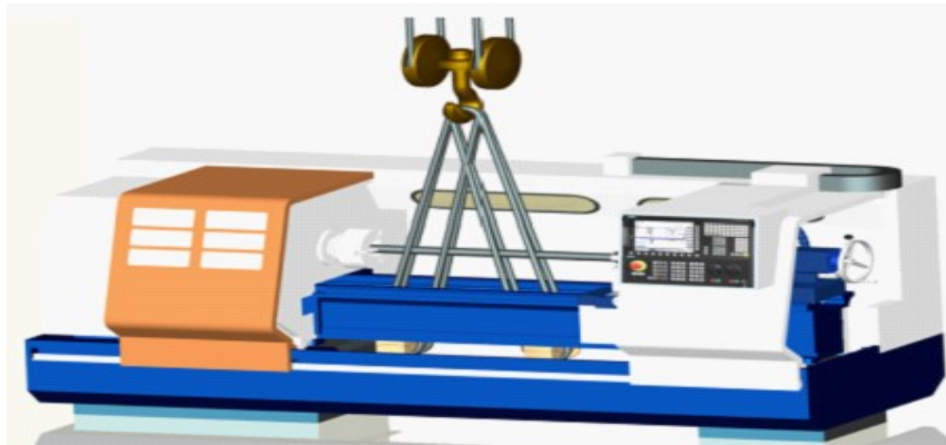
Figure 7.2.2 Lifting drawing of the lathe with center distance is 3000mm
